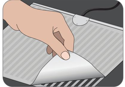
4. Position one edge of the foil on the mirror back, apply pressure evenly as the foil is gradually lowered on to mirror back.
